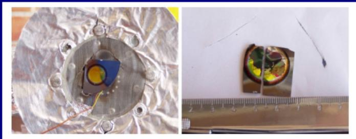
Figure: Porous silicon mirror before and after radiation without cooling
