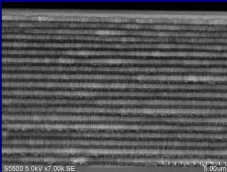
Figure: SEM image of transversal section of a p-Si multilayer
