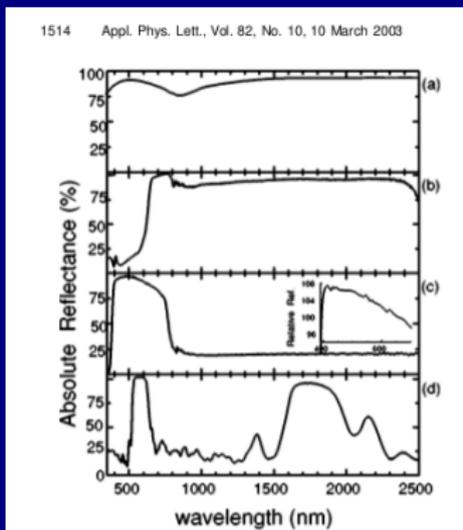
Figure: Reflectance of different porous silicon multilayers
