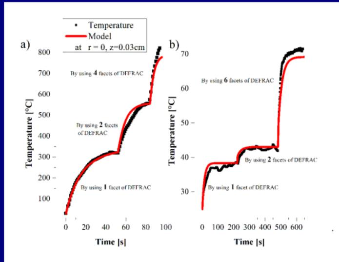
Figure: Time evolution of temperature a) without cooling, b) with cooling
