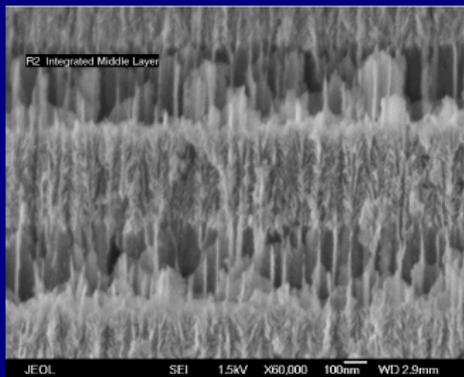
Figure: Nanostructured porous silicon multilayer
