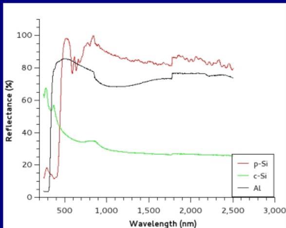
Figure: Reflectance spectrum of p-Si, c-Si and Al mirror
