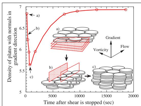
**Figure 2 (right):** The evolution of the small angle neutron scattering pattern from the dispersion with time after a shear of  $1000\text{ s}^{-1}$  is removed (see also front page) [from Brown, Rennie and Clarke].
