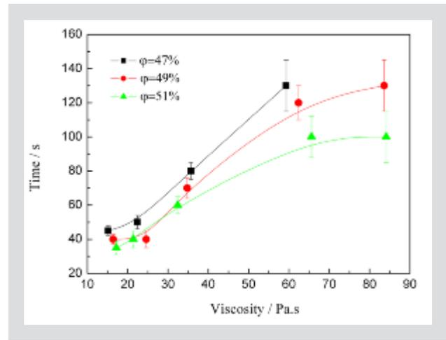
Figure 11: The relaxation time as a function of start viscosity. The volume fraction of suspensions is the 47, 49, and 51 %.
