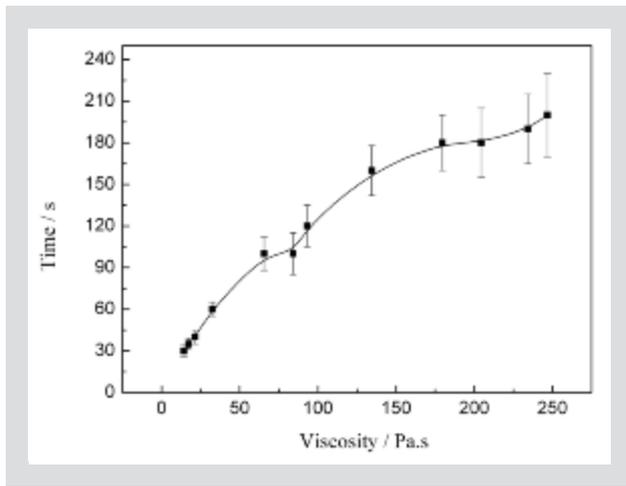
Figure 10: The relaxation time as a function of start viscosity. The volume fraction of suspensions is 51 %.
