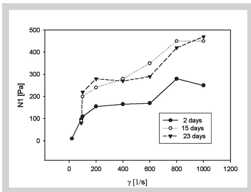
Figure 11: Measurement of viscoelastic properties shows a great scatter of data in low concentrated solutions like in this plot of first normal stress difference,  $N_1$  [Pa], in dependence of shear rate.
