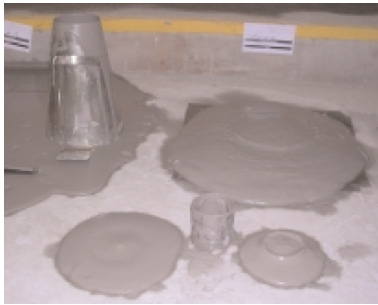
Figure 3: Slump tests during the workshop.
