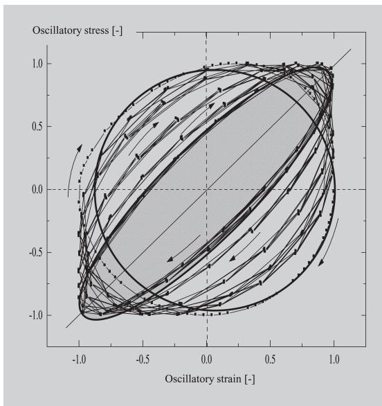
Figure 11: Experimental non-dimensional Lissajous figure for sample S2.
