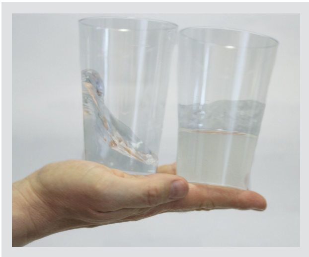
Figure 3: Shaking two partially filled cups of liquid by hand. The left most cup contains water, while the right contains honey thick water. Note that the motion of the surface of the viscous liquid is heavily damped relative to that of the water.
